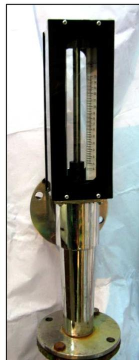
Steel tube flowmeter with magnetically coupled indicator for use with opaque fluids.
