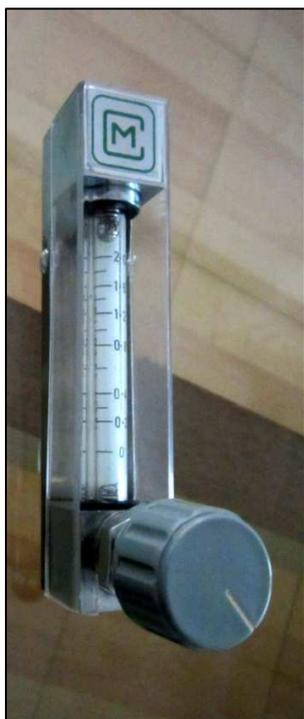
LPG (liquefied petroleum gas) flowmeter customized for range, scale length.
